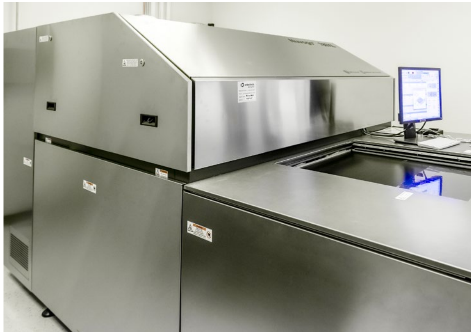
Large format, advanced HDI capable, direct imaging system for outer layers.
